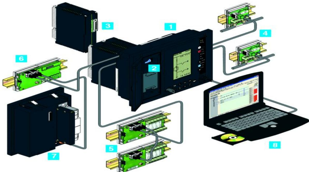
Figure.III.4 : Installation Sepam S80
