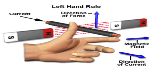
Fig.20 -Fleming's left hand rule
