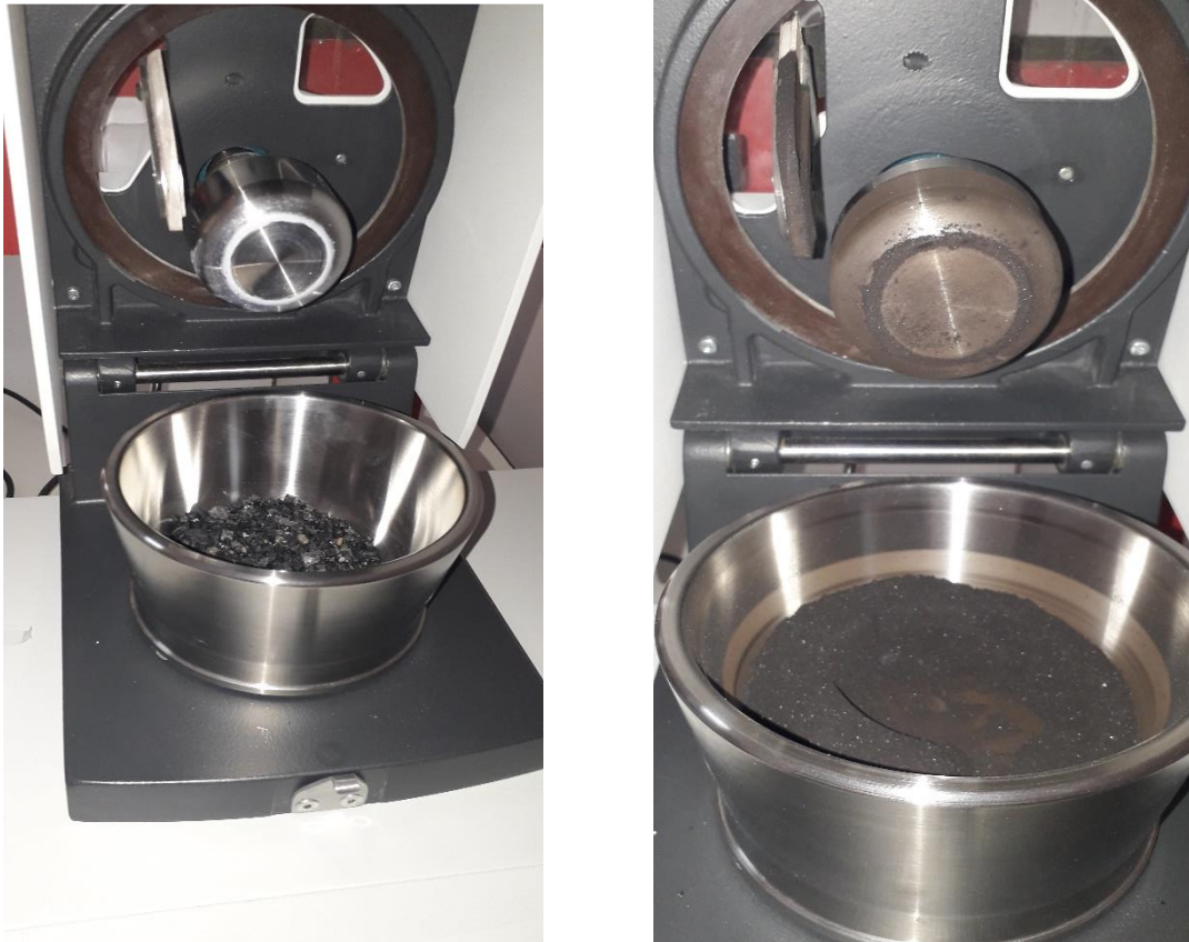
Fig 2 and 3. Raw coal before and after crashing on Jaw crusher.
