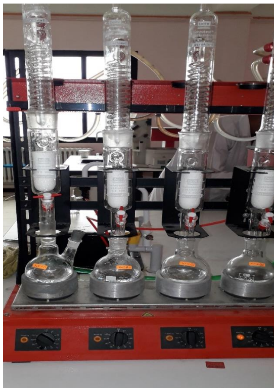
Fig 9. Montage employed for the coal activation process.
