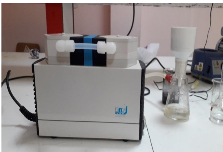
Fig 10 and 11. Filtration of carbon by the Vacuum pump and filter paper.
