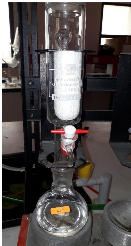
Fig 7 and 8. Activation process by KOH (measure of the agent and assembly used).
