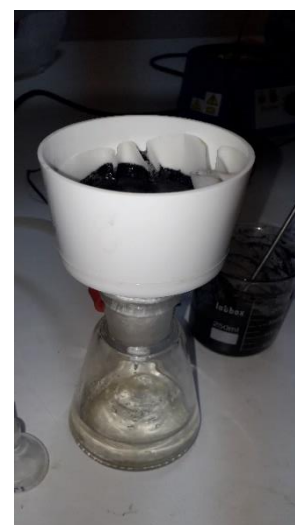
Fig 10 and 11. Filtration of carbon by the Vacuum pump and filter paper.
