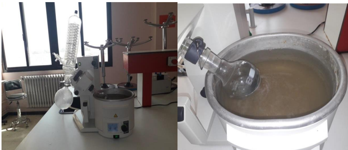
Fig III.3: Elimination of traces of solvent by Rota-vap.
