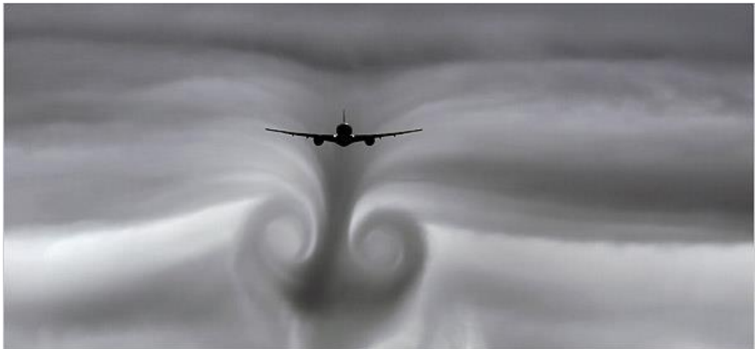
Fig. 2.1 -Turbulence from aircraft swirling clouds below [17].
