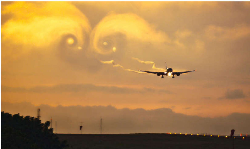
Fig.2.1: Turbulence from aircraft swirling clouds [20].
