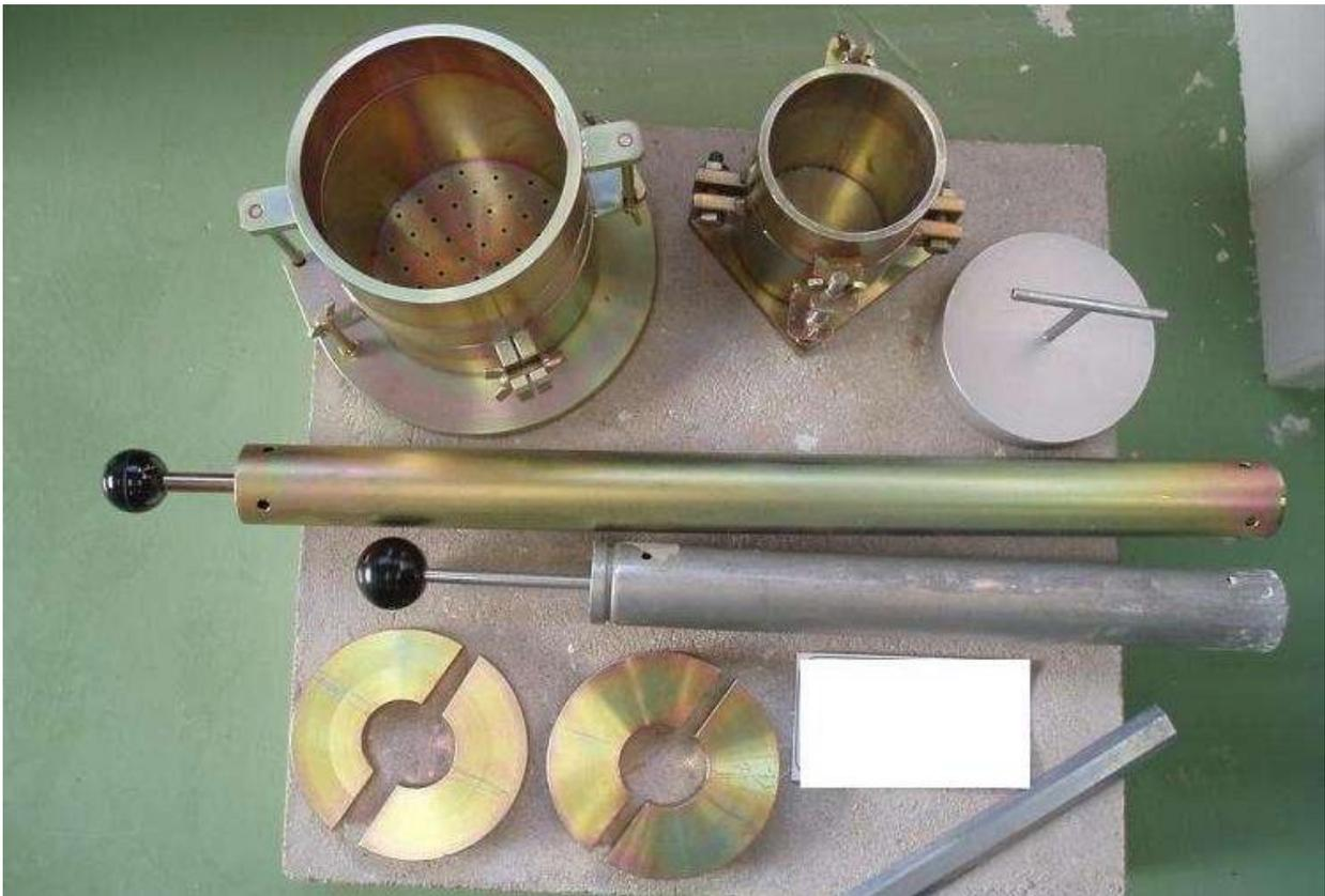
FIGURE 20- MOULE ET APPAREILLAGE PROCTOR CBR
