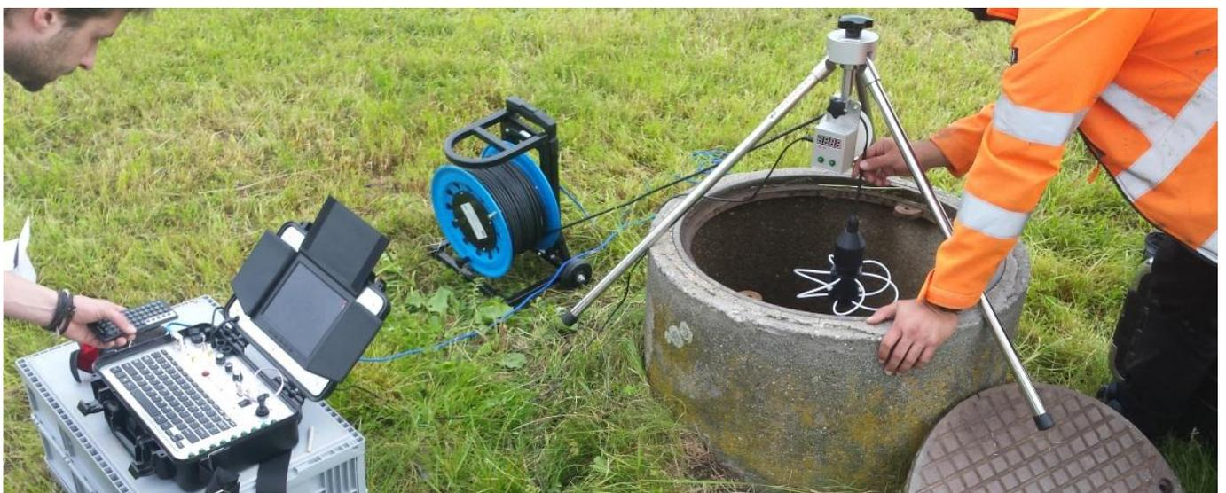
FIGURE 17- ESSAI PIEZOMETRE
