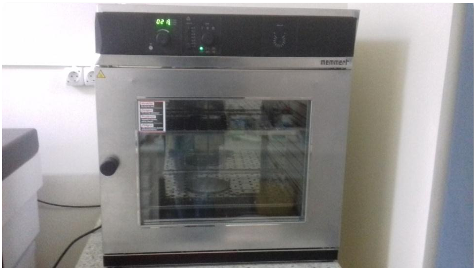
Fig.11. Photo shows the Oven used for drying of the membranes.
