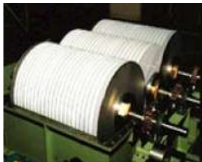
Figure I.23 : Module de Hitachi Rotary Multi-Disk Membrane Separator [47].
