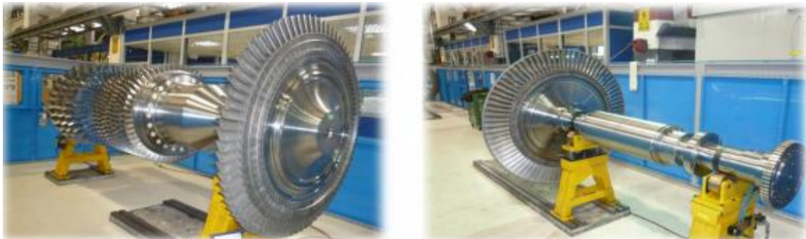
Figure III.10: Turbines HP & BP.
