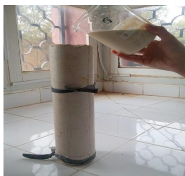
Figure 5.5 : Coulage des supports membranaires
