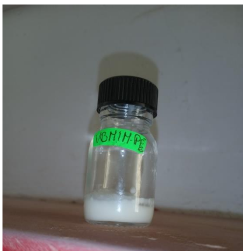
Figure III. 13: 1-méthyl-3-(4-vinylbenzyl) imidazol-3-ium hexafluorophosphate [VBmim-PF 6 ].
