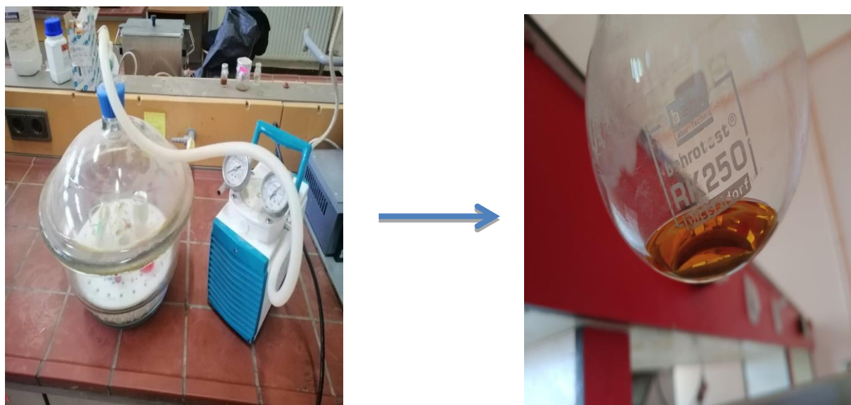
Figure III. 8: Lavage et purification de ([VBmim-NTF 2 ]).
