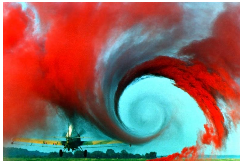
Fig 1- Turbulence from aircraft swirling clouds [19].
