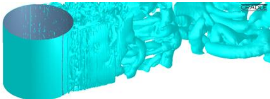
Fig 8 – “DES” simulation of a cylinder above a surface. [35]
