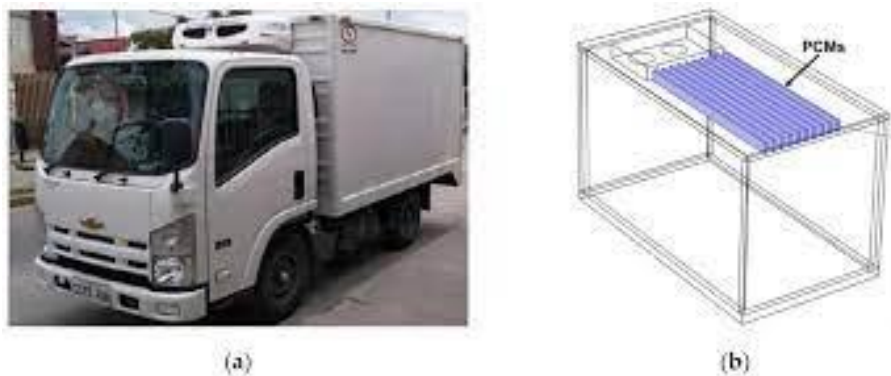
Figure 19-(a) Commercial refrigerated truck; (b) 3D model of the PCM incorporated truck [42]
