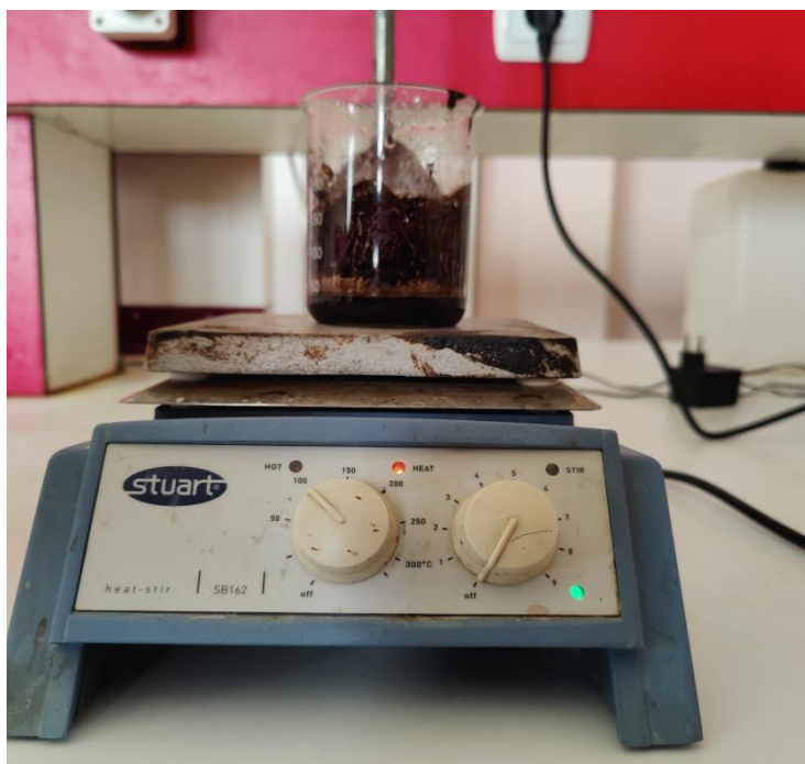
Figure III.15. Photo shows the preparation of copper Nanoparticles gel
