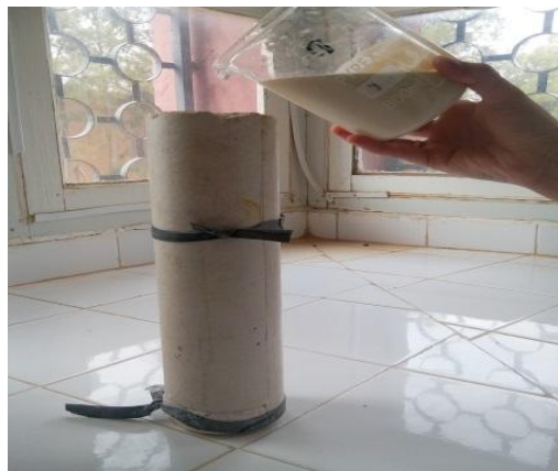
Figure III.4 Casting of membrane supports
