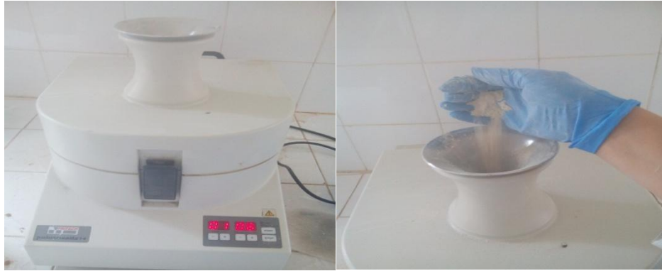
Figure III.2. Mechanical grinding of kaolin
