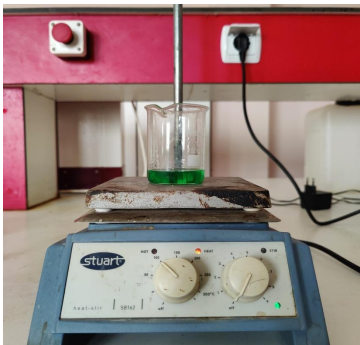
Figure III.11. Photo shows the preparation of Nickel gel
