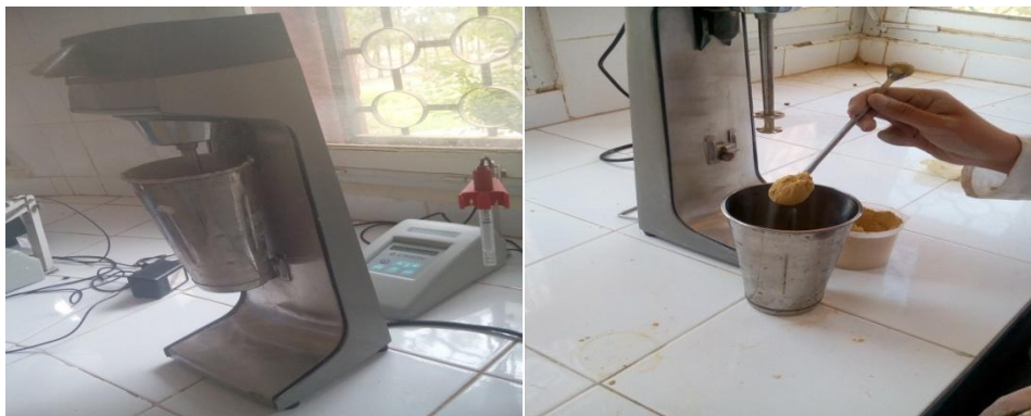
Figure III.3. Preparation of slip for casting
