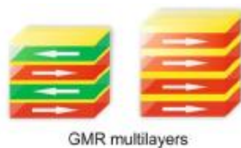
Figure.I.17: Illustration of basic devices for spintronics, GMR multilayers.
