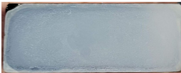
Figure2. 1: Porous thin film of TiO 2 prepared by drop casting on Ge ATR element.
