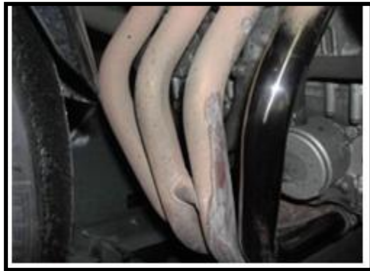
Figure I .7. La corrosion sèche [20]
