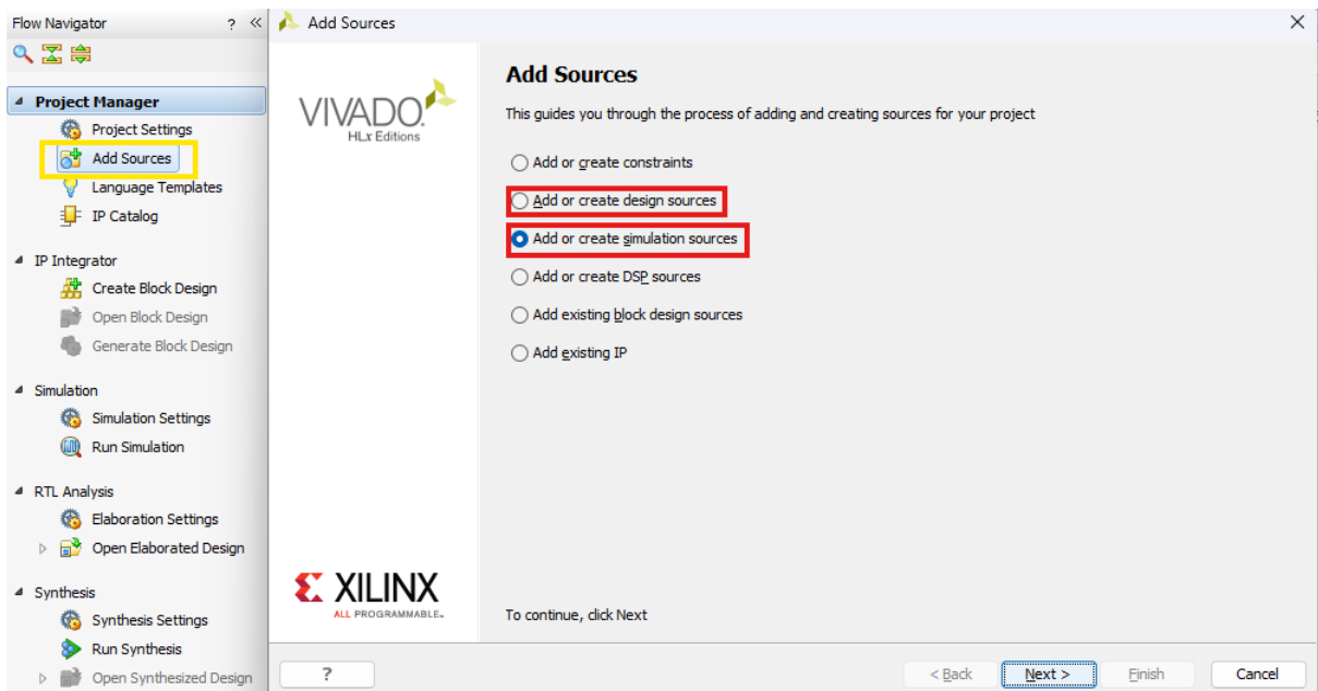
Figure 3.3: Add source in vivado.
