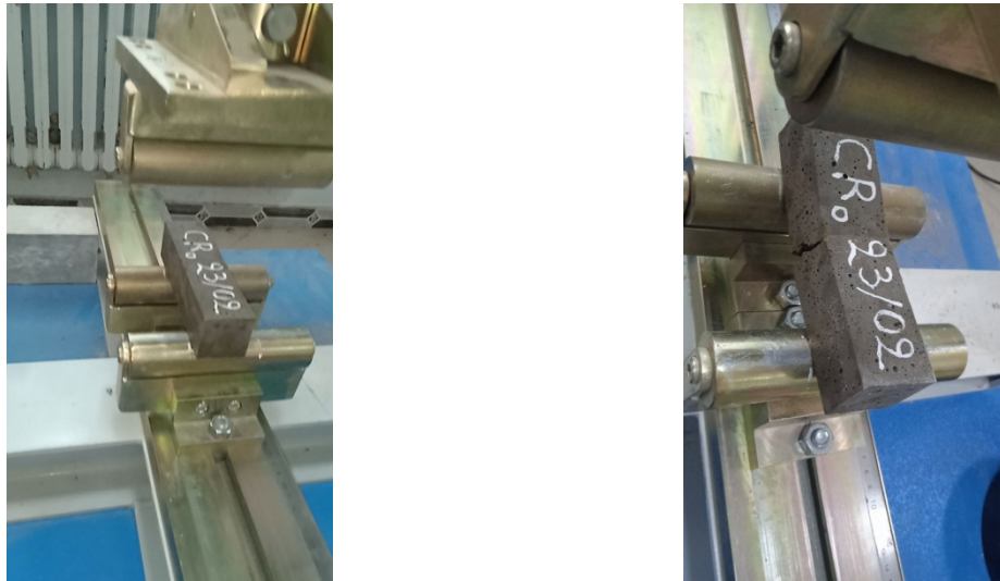
Figure III.17. Flexural tensile test on a mortar specimen.
