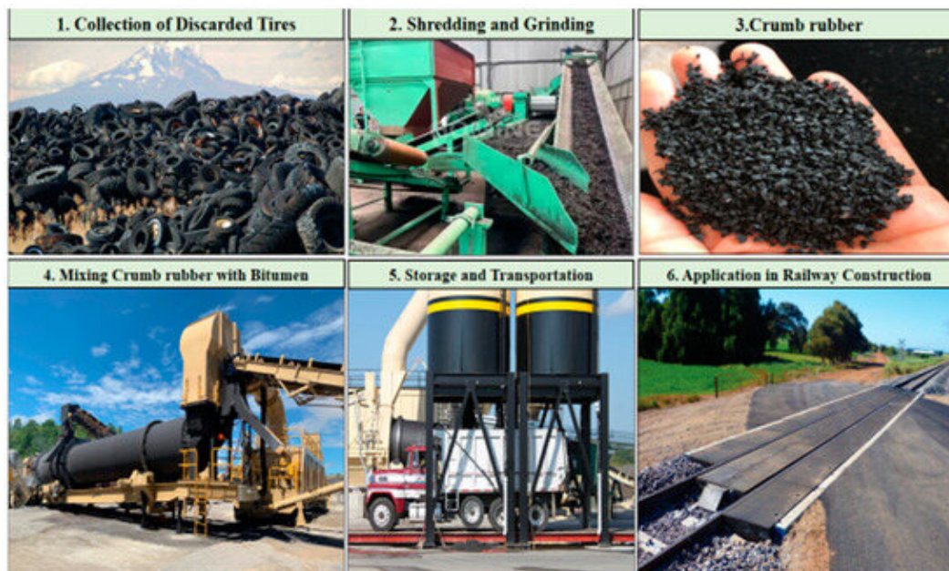
Figure II.5. Processing of waste tires into CR for asphalt application[63].
