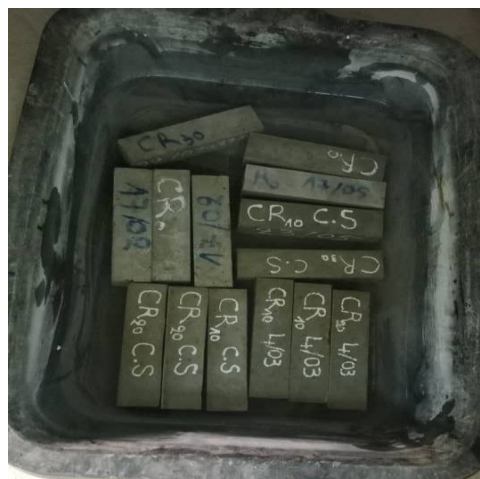
Figure III.15. Curing tank for the different specimens
