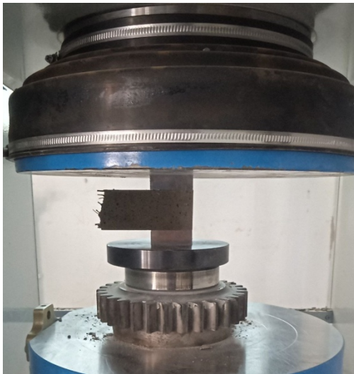
Figure III.18. Compression test on a mortar specimen.
