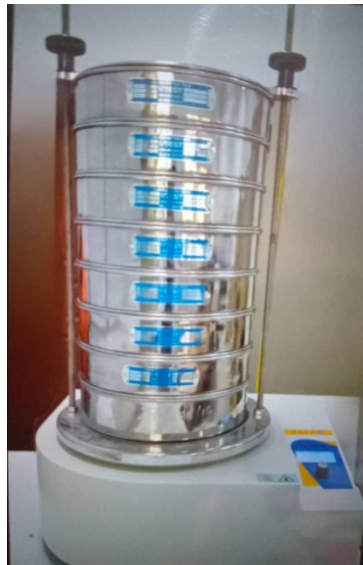
Figure III.5. Sieve used to determine the granulometry of sands.
