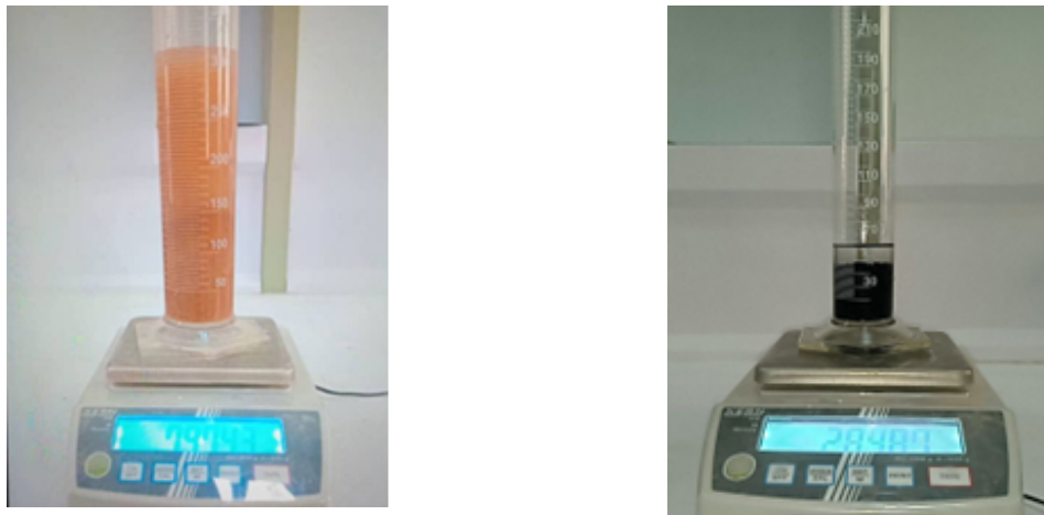
Figure III.8. Method used to determine the absolute density of a sand.
