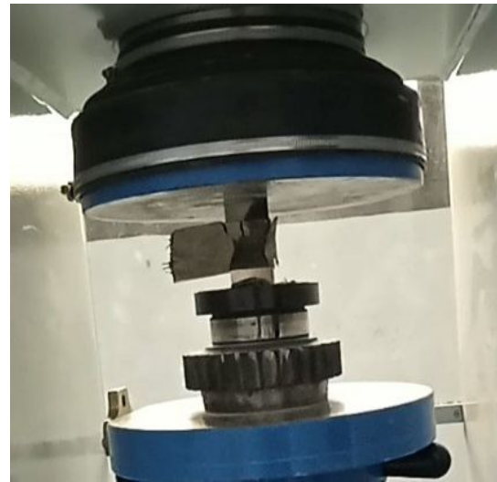
Figure III.18. Compression test on a mortar specimen.
