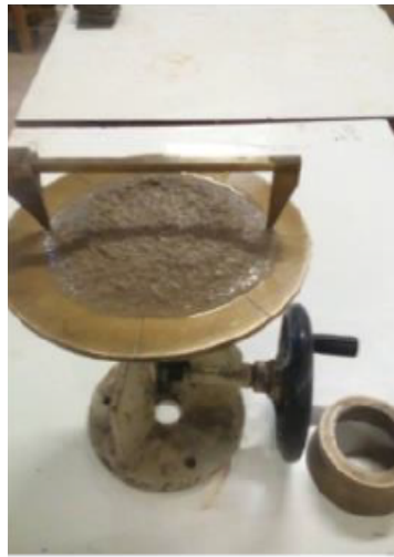
Figure III.12. Spread test for mortar
