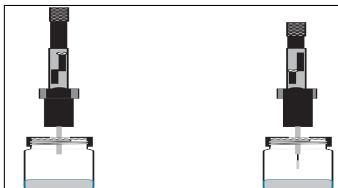
Figure 73. Solid Phase Microextraction (SPME) showing the fiber in the raised and lowered positions.
