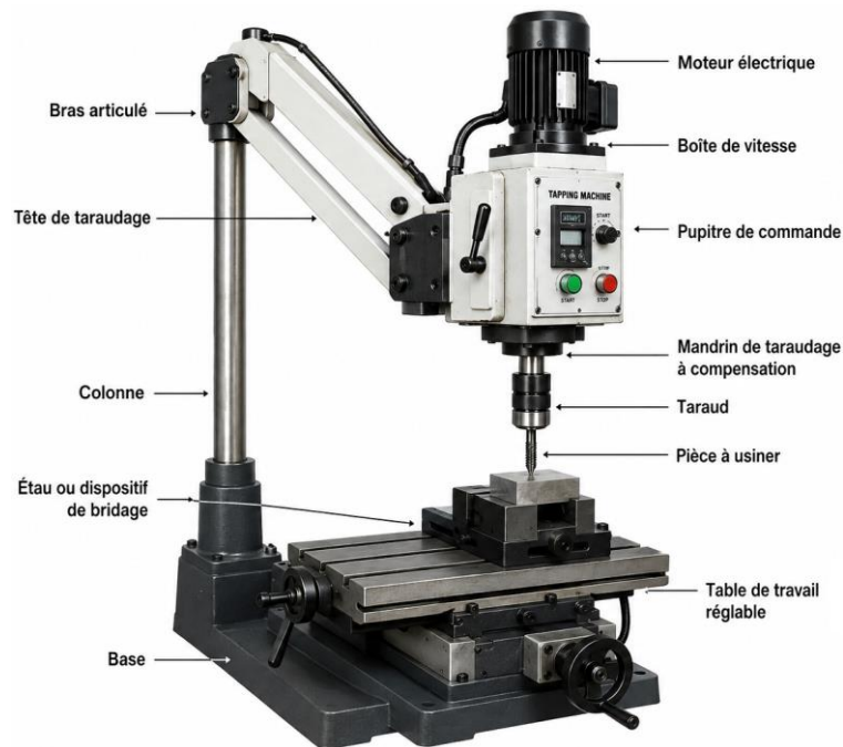
Fig.1-20 Machine de taraudage [8].
