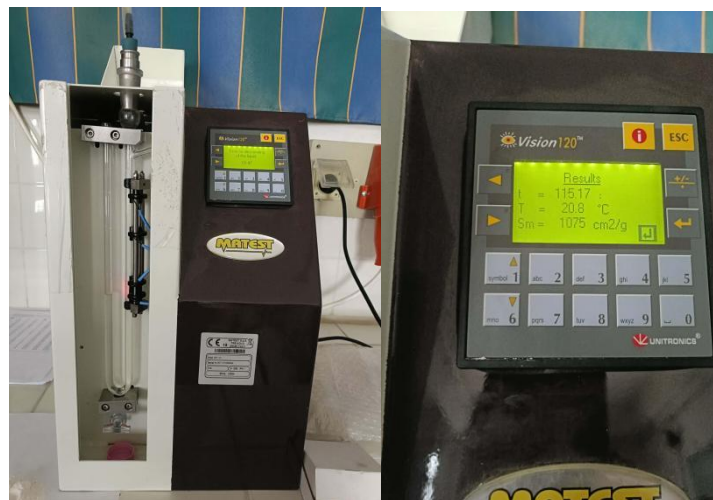
Figure III.8 Measurement of TAMP fineness using an automatic Blaine air-permeability apparatus.
