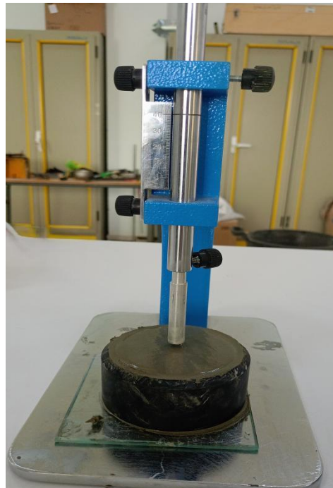
Figure III.11 Vicat apparatus used for determining the standard consistency and setting time of the binder pastes.
