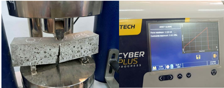
Figure III.13. Three-point flexural tensile strength testing configuration on a 4×4×16 cm mortar prism specimen
