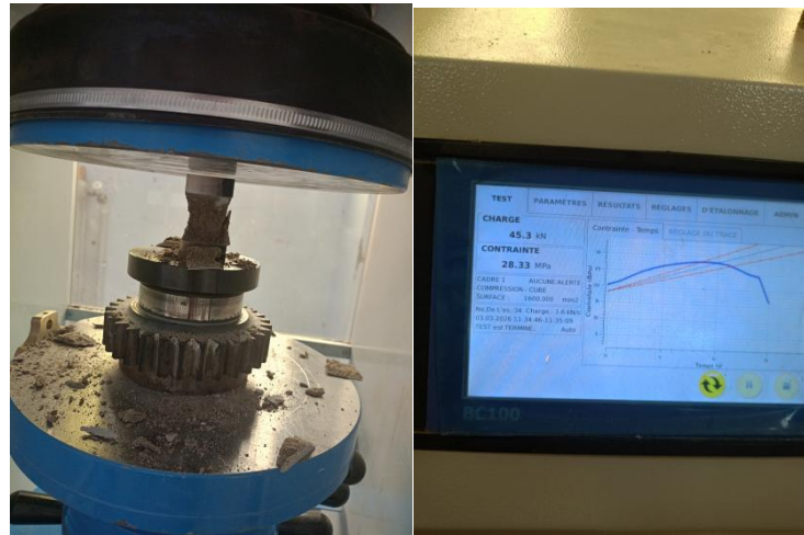
Figure III.12 Hydraulic press displaying failure load and stress-time curve during compression testing
