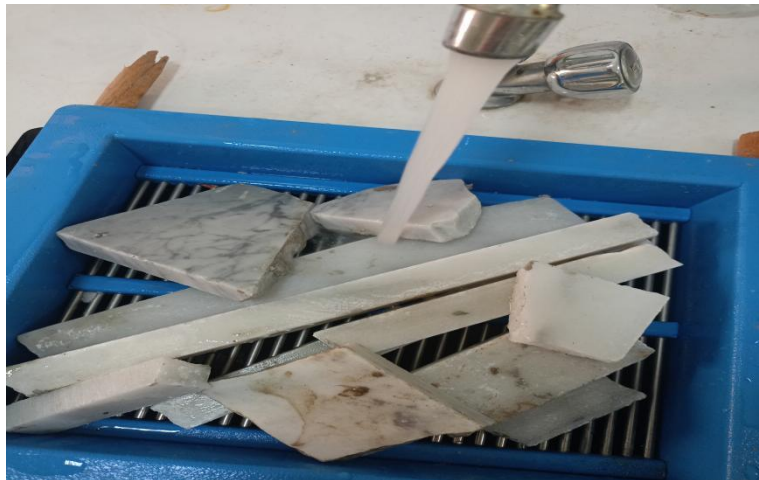
Figure III.5 Raw Carrara marble waste fragments during the cleaning process.
